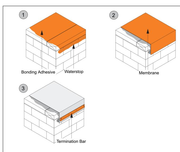
1. Apply Bonding Adhesive to the clean substrate and to the back of the membrane. Allow to flash off. While the Bonding Adhesive is flashing off, apply a 3/8" bead of Waterstop below the bottom of the deck or nailer.
