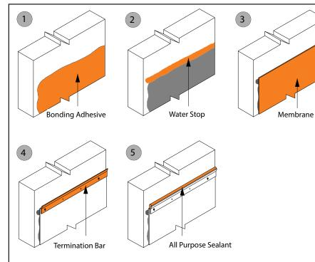
1. Apply Bonding Adhesive to the clean substrate and to the back of the membrane flashing. Allow to flash off.
