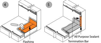
Note: Peel and Stick TPO membrane has factory applied adhesive on the back of the sheet, eliminating the need for application of Bonding Adhesive as shown above. In lieu of applying Bonding Adhesive to the substrates, apply All Purpose Primer, and allow it to flash off completely prior to installing the Peel and Stick TPO membrane.
