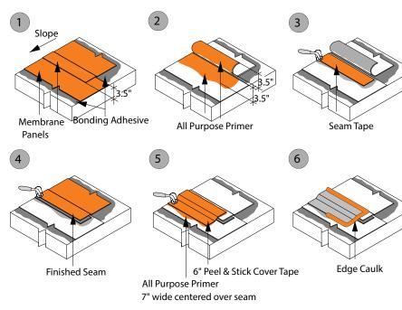
1. Align adjacent membrane panels to achieve a 3-1/2" wide overlap with the top panel being up slope of the lower panel and bond to the substrate.
