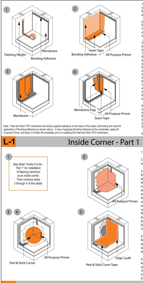
1. Measure the area to be flashed from the intended flashing height to the deck and into the field 3" and cut flashing membrane to size accordingly.
