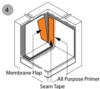
Note: Peel and Stick TPO membrane has factory applied adhesive on the back of the sheet, eliminating the need for application of Bonding Adhesive as shown above. In lieu of applying Bonding Adhesive to the substrates, apply All Purpose Primer, and allow it to flash off completely prior to installing the Peel and Stick TPO membrane.
