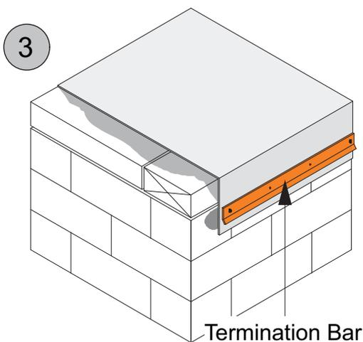
1. Apply Bonding Adhesive to the clean substrate and to the back of the membrane. Allow to flash off. While the Bonding Adhesive is flashing off, apply a 3/8" bead of Waterstop below the bottom of the deck or nailer.
