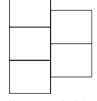
Always stagger insulation joints, regardless of board size used.
